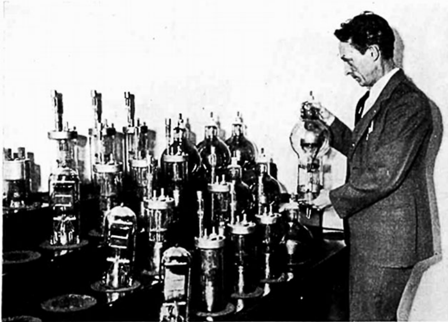
This display rack contains (left to right) 4 250-watt modulators (Western Electric type 212-E), 11 35 kw. r-f amplifiers (W. E. 232-A), and 7 10-amp. mercury rectifiers (W. E. 266-A), spares for the new 50-kw. WOR transmitter at Carteret, N. J.
