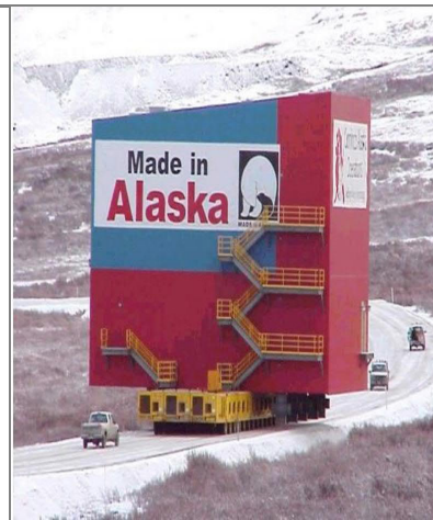
Figure 3 Red Dog Lead-Zinc Flotation module on the move. 114' x 64' x 75' high, weight 1,600 tons, Courtesy Red Dog Mine.
