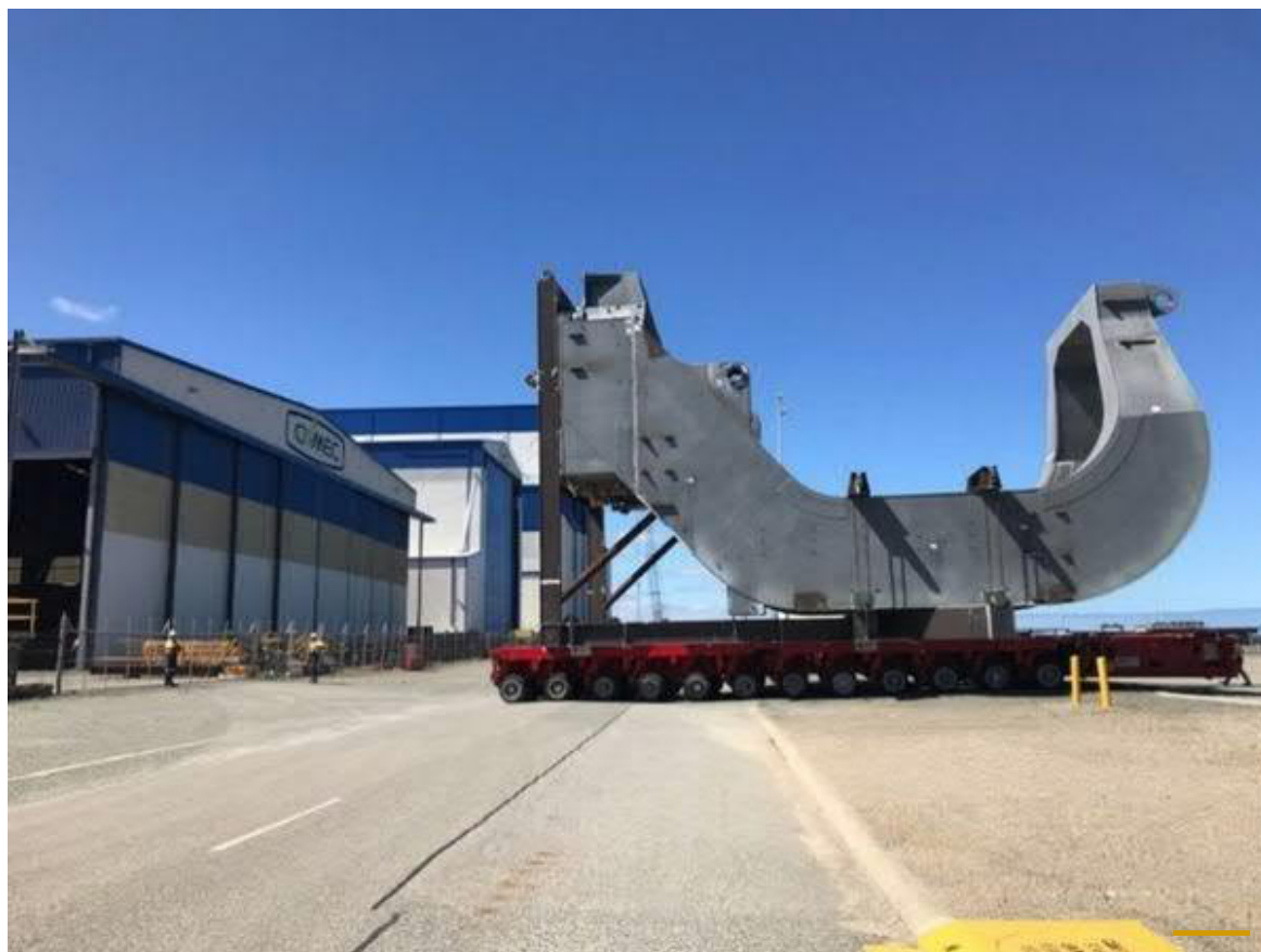
Figure 7 South Flank Mine Modular Bracket part being moved out of factory. Courtesy of Civmec
