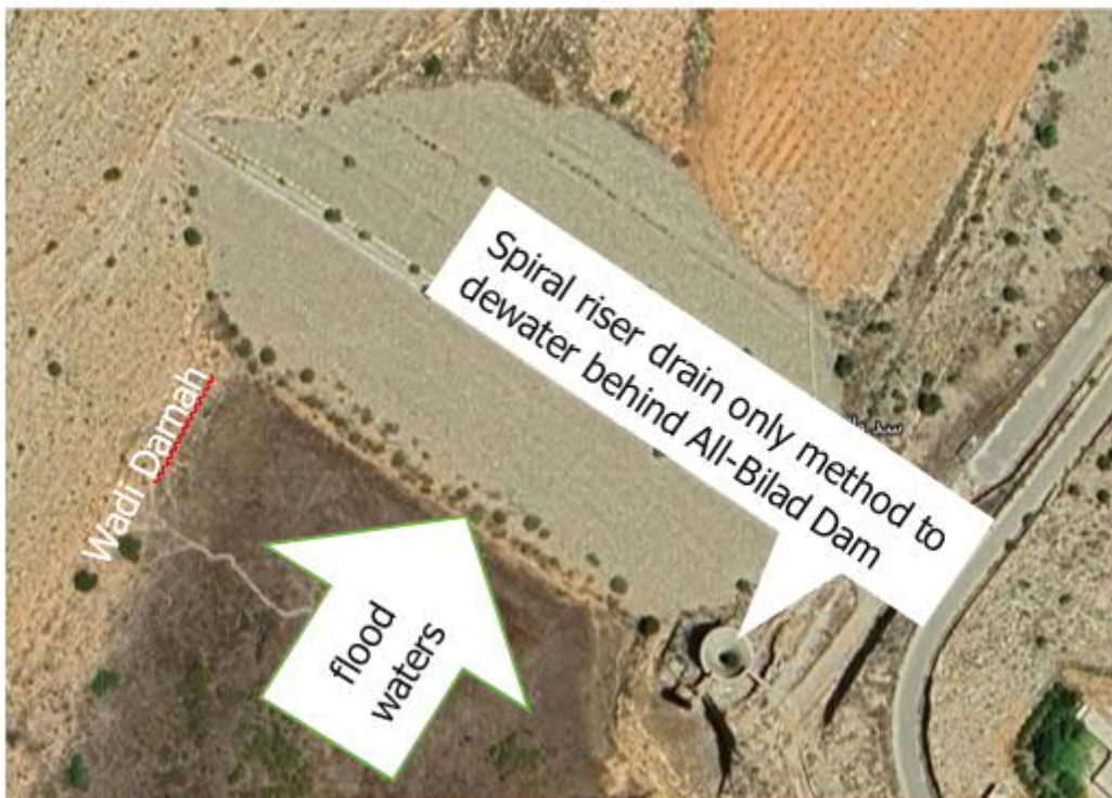
Figure 2 Upper Al-Bilad Dam failed first September 10 along Wadi Darnah. Dam had a spiral riser pipe, with no emergency spillway. Author's figure. Google Earth
