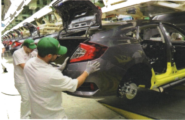
A rear bumper fascia is installed at Honda of Canada Mfg.
