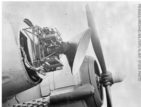
Microwave radar enabled the Royal Air Force Bristol Beaufighter Mk. VI to intercept inbound German bombers at night.
