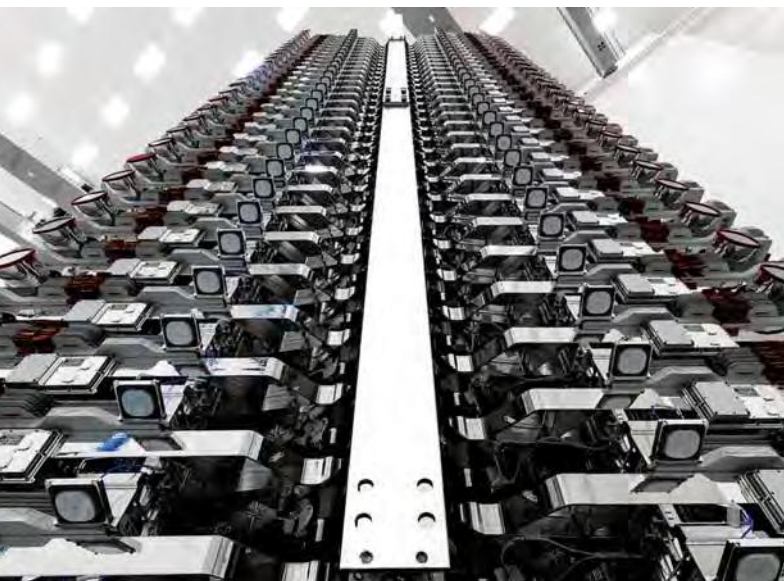
▲ LOCKED AND LOADED Sixty Starlink satellites are packed like sardines within the nosecone of a SpaceX Falcon 9 rocket.
