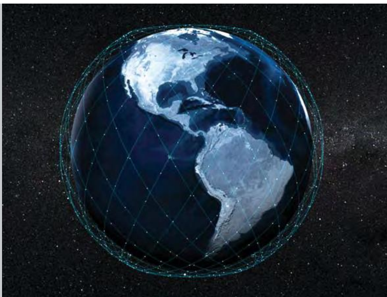
▲ GLOBAL PRESENCE This image shows the initial phase of the Starlink constellation: 1,584 satellites in 24 orbital planes at 550 km. (SpaceX has applied to the FCC for a change to this configuration, spreading the same number of satellites across 72 planes.)
