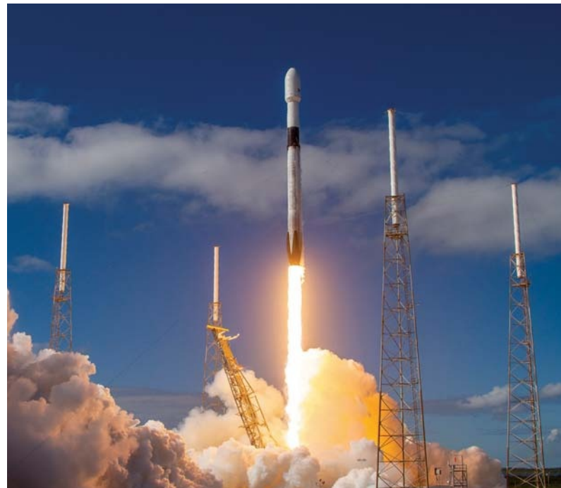
▲ 10, 9, 8 . . . Sixty Starlink satellites launched on May 23, 2019, aboard a Falcon 9 rocket. Another packet of 60 launched on November 11th, shown here. The May launch deployed to an altitude of 440 km and the November launch to 280 km, but both sets of satellites will operate from 550 km.
