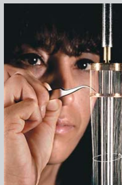
SCIENTIST builds an array of wires for the Z Machine.
