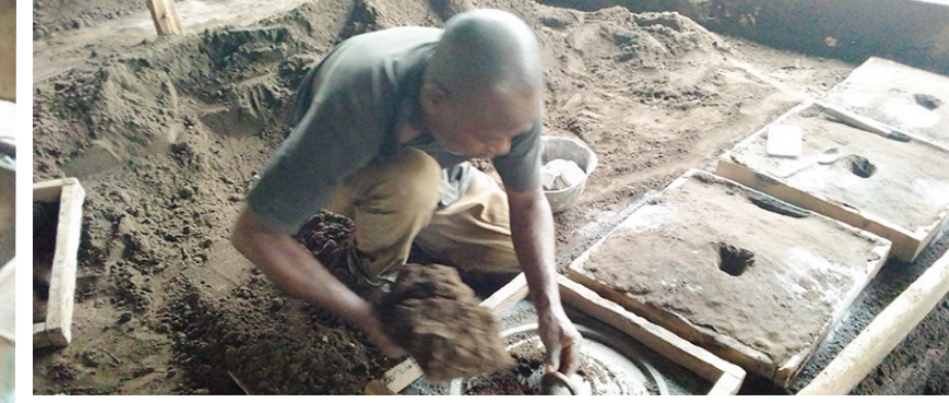
The pots and the lids are moulded concomitantly. Powder enables the free circulation of the melted metal
