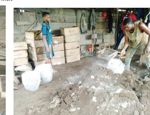
After about 10 minutes, the melted metal in the boxes are transformed into aluminium pots
