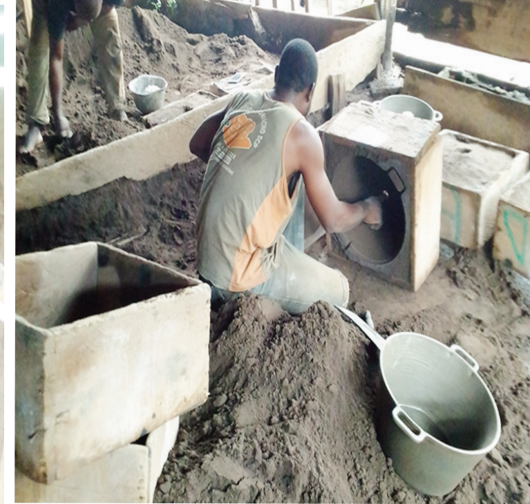
A mixture of soil and sand, as well as a box are used to form the prototype of the pot
