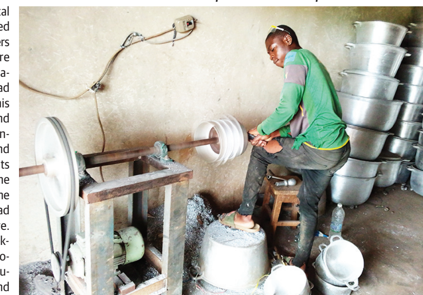
The pots are sandpapered to ensure smoothness
