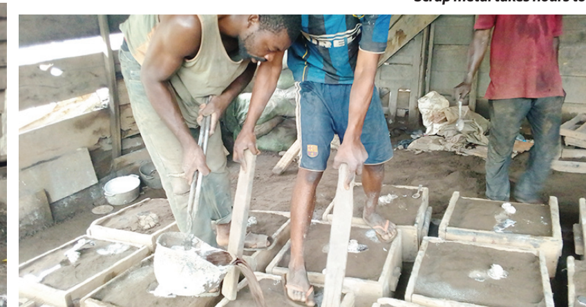
The melted metal is poured into the prototypes to form aluminium pots
