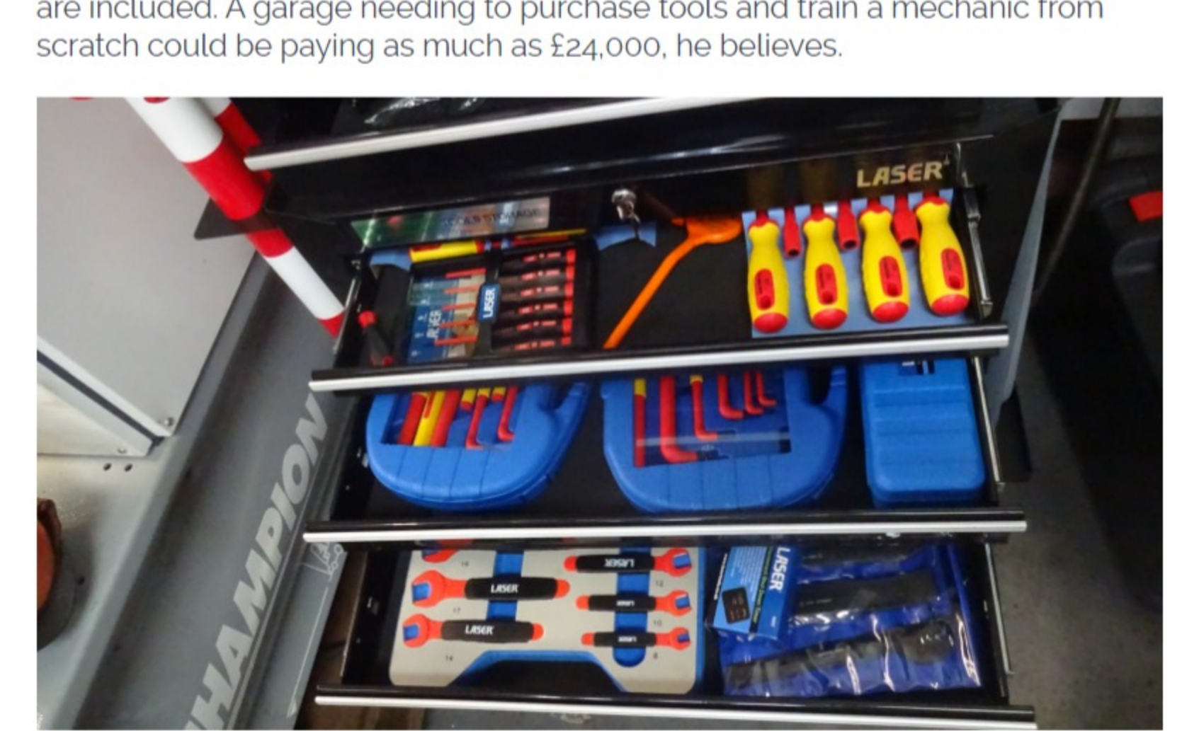
A selection of specially insulated tools required to work on electric vehicles.
